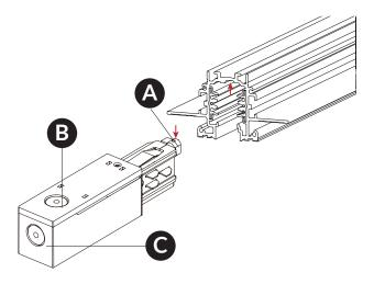
In order to correctly wire the system, the End Feed has a mechanical key / groove (A) that ensures the correct insertion into the track. When installing, ensure that the mechanical key is oriented properly.
